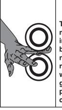
**A** CAUTION The main rollers of this machine present a pinching hazard. Make sure no body part or clothing is near the area between the rollers. Failure to follow this warning may result in fingers, hair, or clothing being pulled into the machine, causing personal injury.
